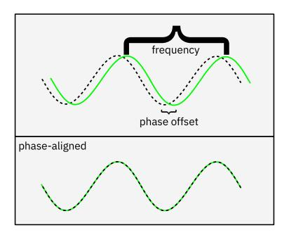
The following diagrams help describe how phase error of the contour generator (in green) changes over time relative to the input clock. The vertical lines are points where phase adjustments can occur and the dashed line represents an input clock. Depending on the given ratio, this may happen on every rising edge of the input clock, or once every N cycles.
