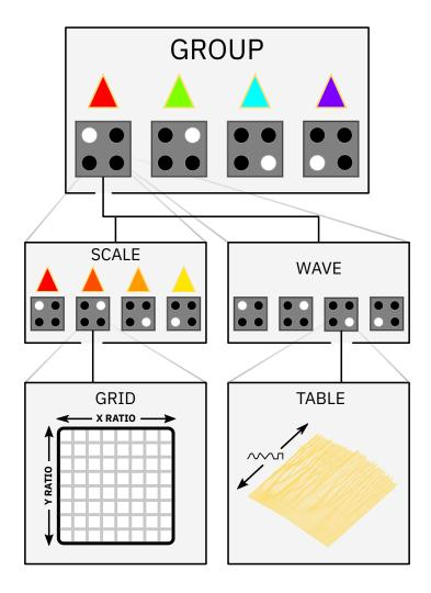
The first group is organized with an ascending numerator on the X axis (steadily increasing frequency multiplication) and an ascending denominator on the Y axis (steadily increasing frequency division). The available tables are appropriate for use as control voltages or audio signals.
